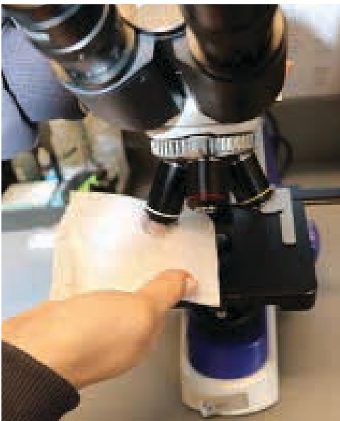
Once focused on 40x move objective slightly, put a small drop of oil on the slide then move the oil objective toward the slide and focus.
