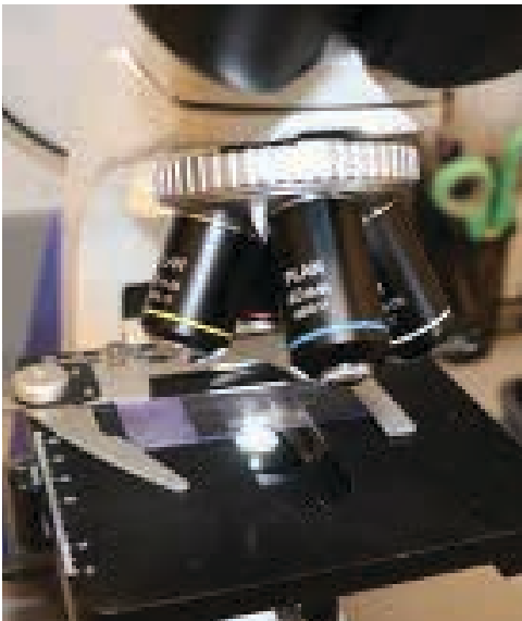
Place slide on stage, focus on 10x first.
