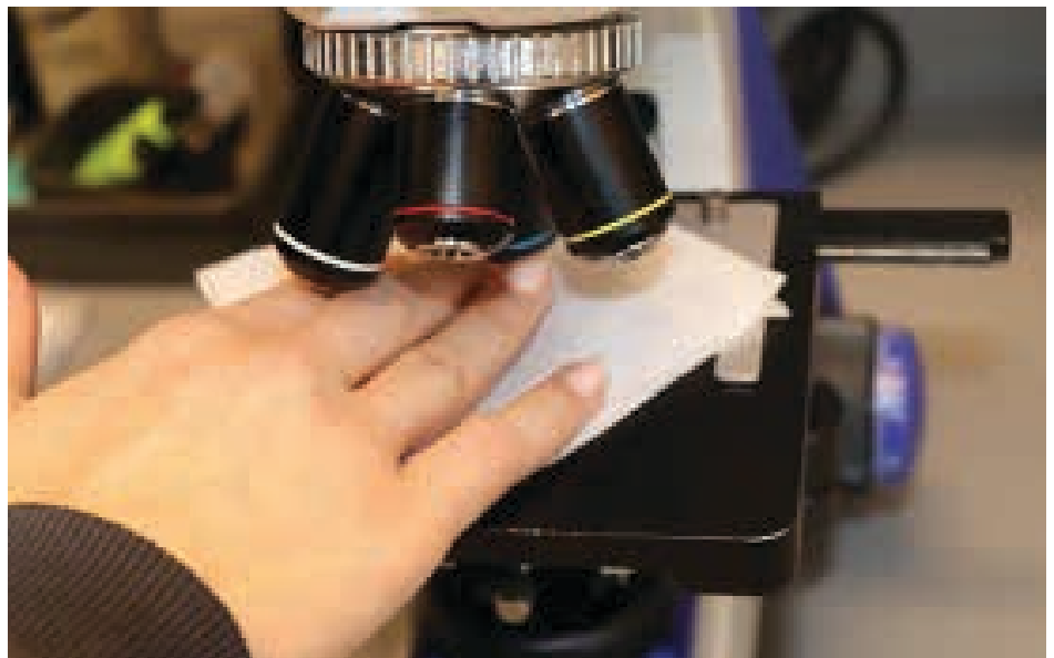
Once focused on 40x move objective slightly, put a small drop of oil on the slide then move the oil objective toward the slide and focus.
